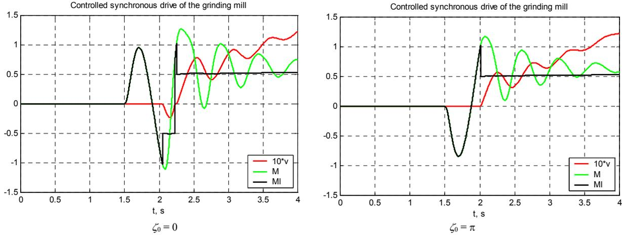
Fig. 3. Processes of drive model for two values of initial angle  $\zeta_0$  between currents vector and  $d$  axis of motor:  $v$  – velocity,  $M$  – motor electromagnetic torque,  $M_l$  – load torque (relative values)
