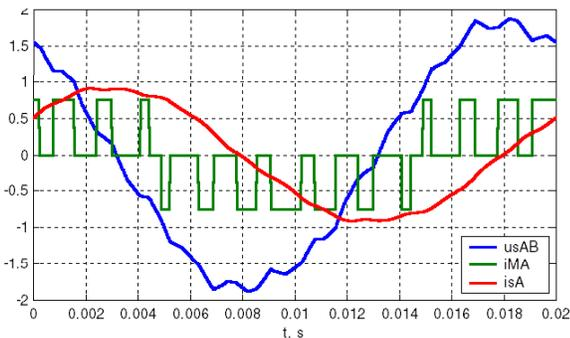
Fig. 2. Operation principle of a PWM CSI:  $iMA$  - output current of converter,  $usAB$  - stator line-to-line voltage,  $isA$  - stator current (relative values)
