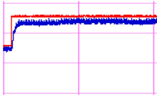
Fig. 4. Ball mill drive. Response of current control loop. Reference step for DC link current:  $I_{DG}(0) = 0.4$ ,  $\Delta I_{DG} = 0.2$  (relative values). Time grid division – 0.1 s
