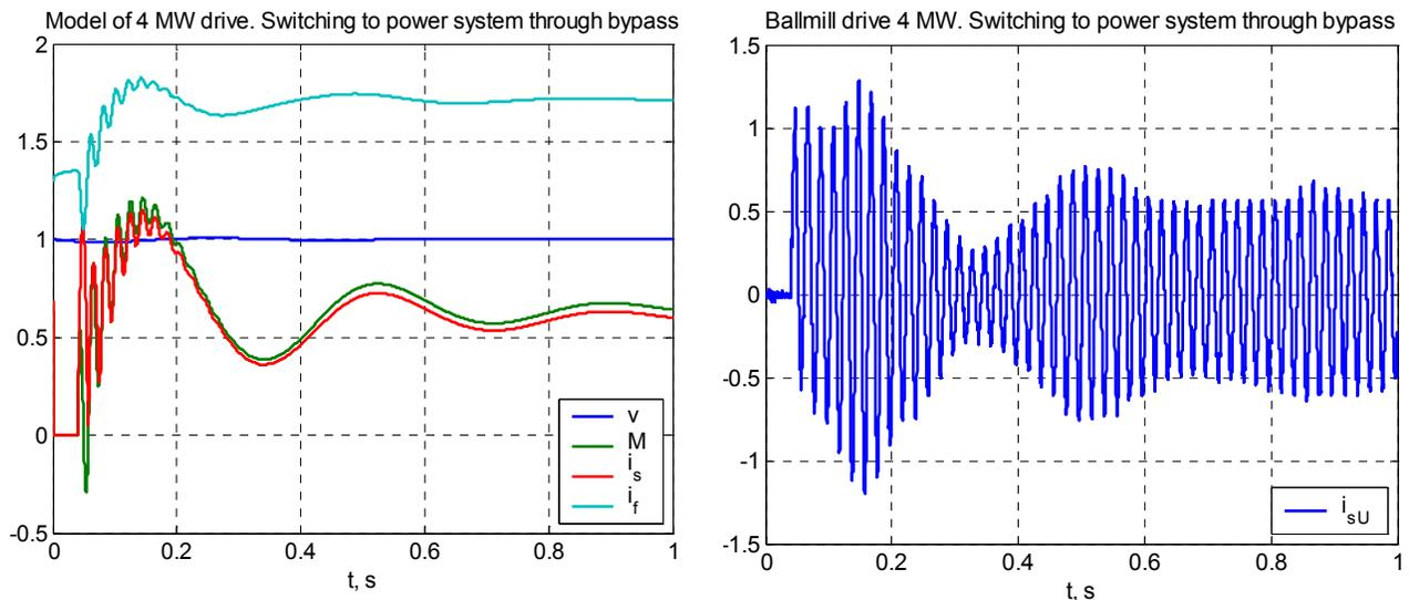
Fig. 6. Processes of drive model and real drive while switching to power system:
