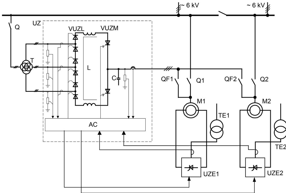
Fig.1. Functional diagram of the drive system:  $M1, M2$  – motors,  $UZ$  – CRD,  $T$  – transformer,  $UZE1, UZE2$  – exciters,  $TE1, TE2$  – transformers of exciters,  $Q, Q1, Q2, QF1, QF2$  – contactors,  $VUZL$  - line converter,  $VUZM$  – machine converter,  $C$  – filter capacitor,  $L$  – DC link reactor,  $AC$  – automatic control device
